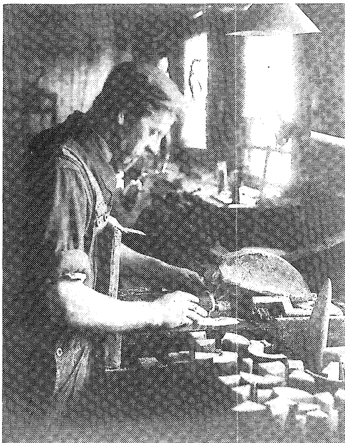
Figure 9. A sawyer at Wood & Brooks (Buffalo) parting junked tusk sections into head and tail blocks. Semi-sawed blocks stand in the foreground. Note coolant shields over saw blade and sawyer's chest. Wood & Brooks Records Collection (457), Archives Center, National Museum of American History, Smithsonian Institute.
